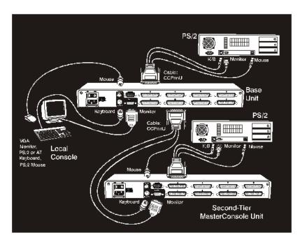
Figure 19 Two-Tier Configuration Cabling Detail
